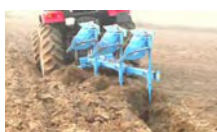
Super power ploughing with reversible MB plough
