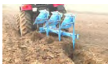
Super power ploughing with reversible MB plough
